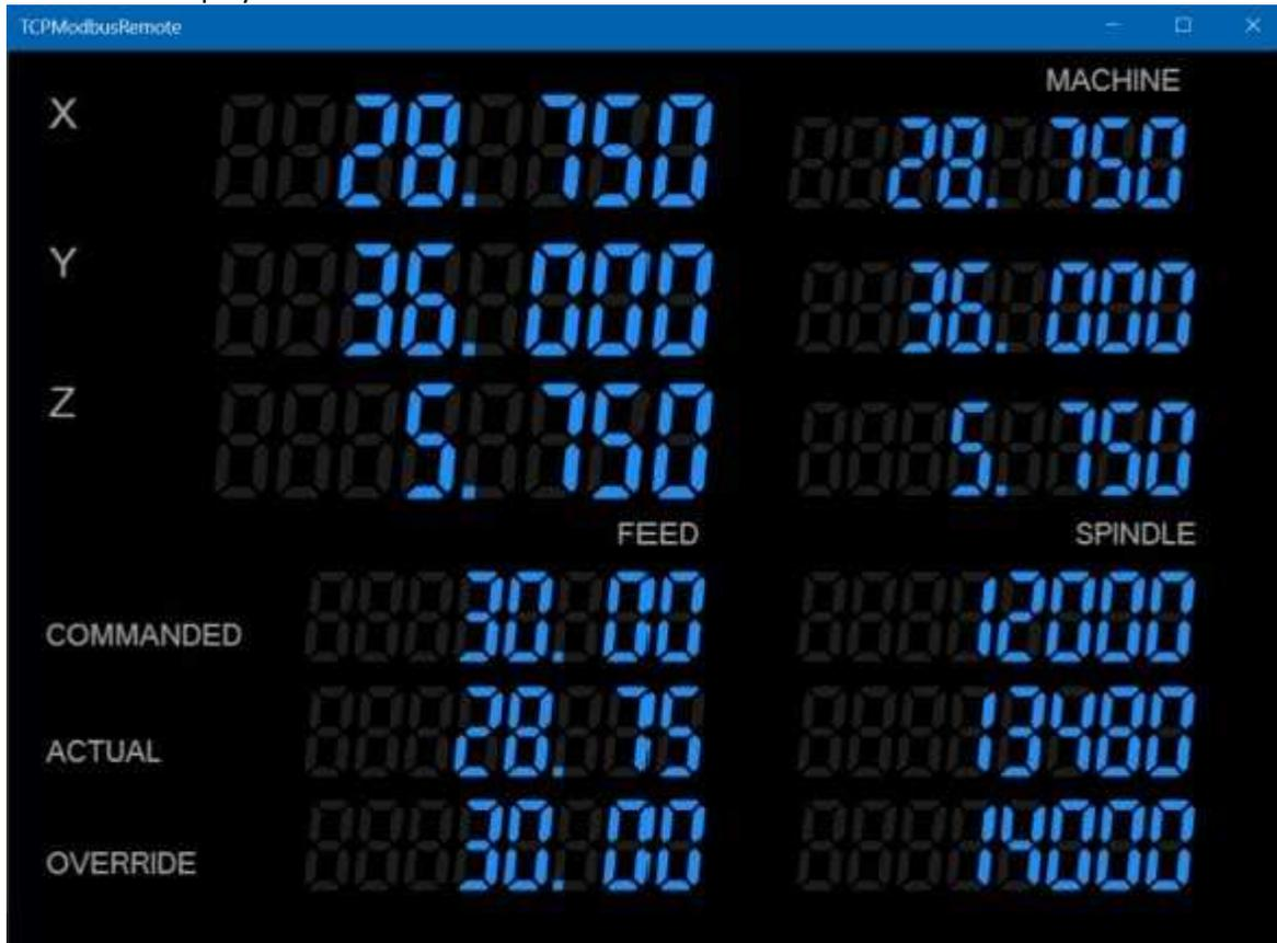
Set the IP address to the machine running the remote DRO software. It can also be on the the same machine running UCCNC for testing. Run 'cmd' and type 'ipconfig /all' if you don't know the machine's address.
