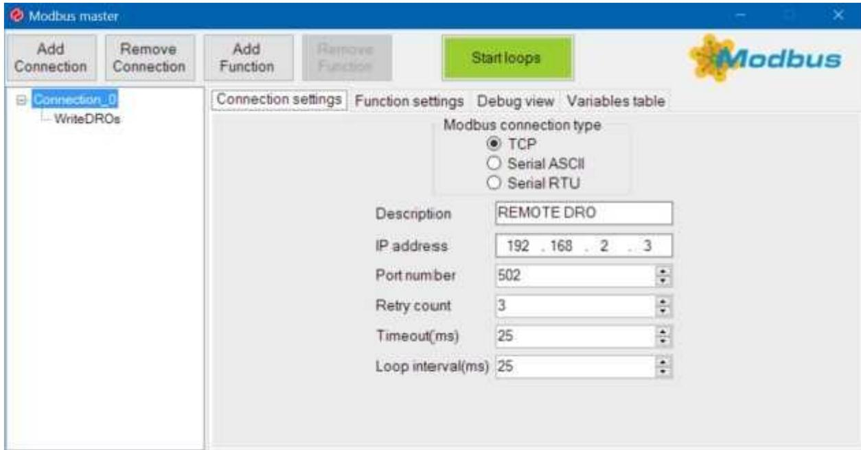
A function to write the values must be created. Register count must be 24 for the current macro
